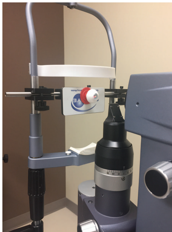
Figure 1. Example of laser simulation setup with the SimuleYE slit lamp holder and SimuleYE LPI model eye.
